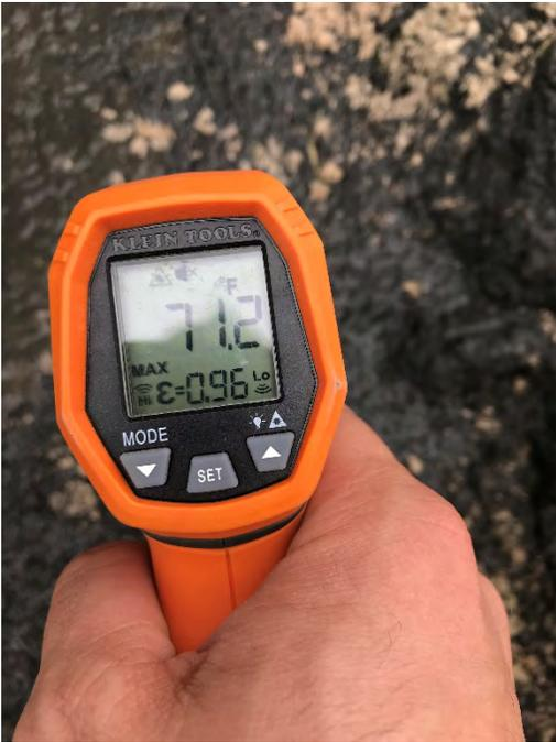
Photo 2: IR gun utilized to assess temperate of un-amended sediment.
