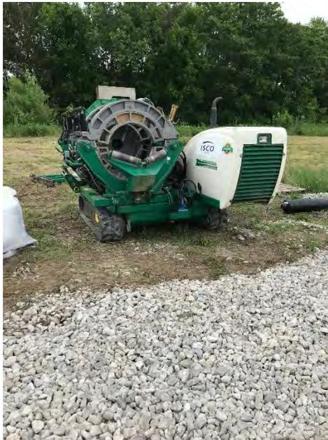
Photo 1: Butt Fusion Welder
