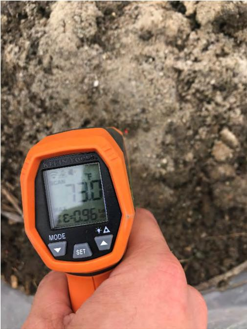
Photo 1: IR gun utilized to assess temperature of amended sediment.
