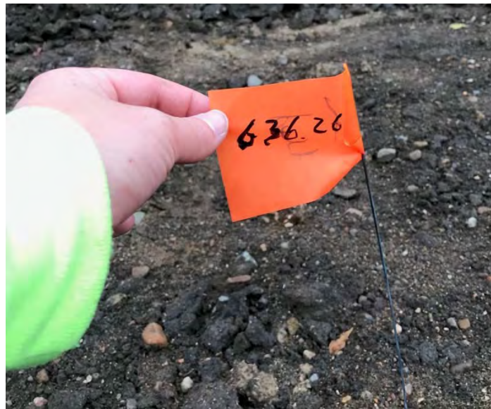
Photograph 1 – Surveyed bottom elevation in Area H.
