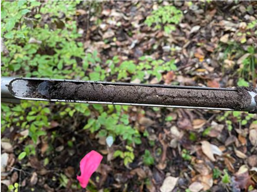
Photo 5: Soil core recovery to assess depositional feature.
