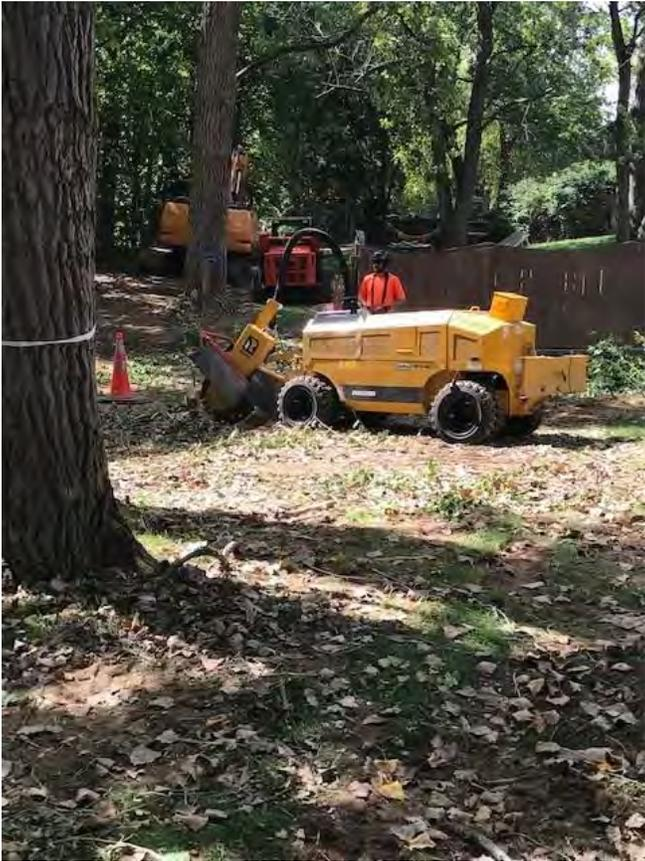
Photograph 2 – TNT performing stump grinding of large stumps
