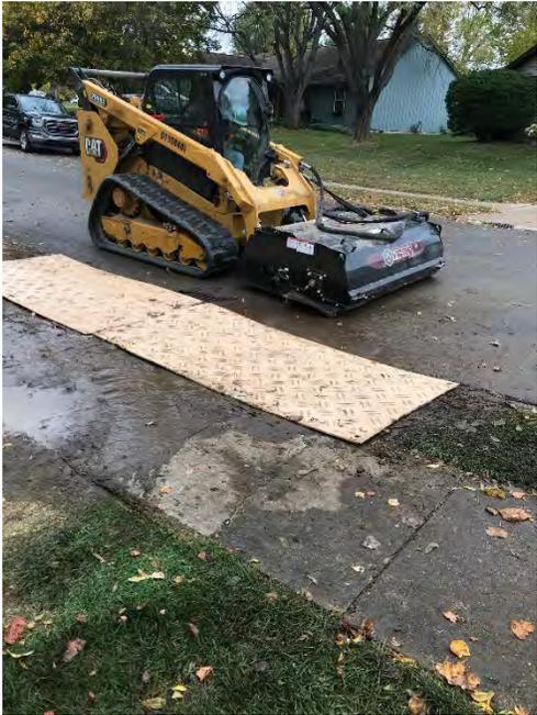
Photograph 3 – Skid-steer with street sweeper attachment cleaning the Windmill Drive entrance.
