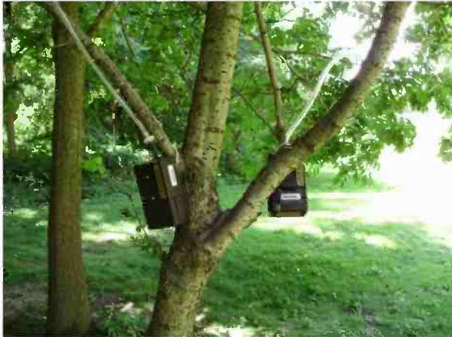
**Air monitoring equipment set up at the perimeter of the work area.**
