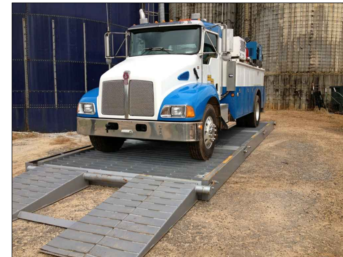
TRACTOR DRY WHEEL WASH SYSTEM BY INNOVATIVE EQUIPMENT SOLUTIONS (PICTURED) OR APPROVED ALTERNATIVE TO BE IMPLEMENTED AT SITE EXIT
